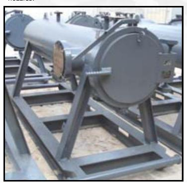
WARCO also offers economical single element vessels for less flow rates. Both horizontal and vertical vessels are available. An 8" diameter WARCO vessel containing a single 80" filter can handle up to 500 gpm flow and match the solids holding of a larger 24" diameter vessel with standard 40" depth filters.
