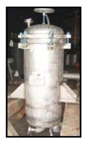
Vertical vessels are also an option for 40" High Capacity Filters. Existing cartridge and bag filter vessels can be upgraded to WARCO High Capacity Filters with minimal changes to existing piping and foundation.
